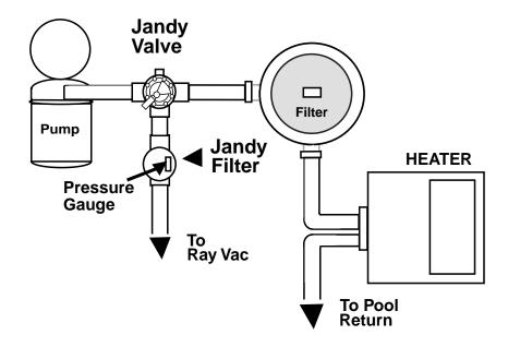
After the Jandy Valve and Energy Filter have been plumbed, install the Pressure Gauge in top of Energy Filter. Use the teflon tape and hand tighten.
