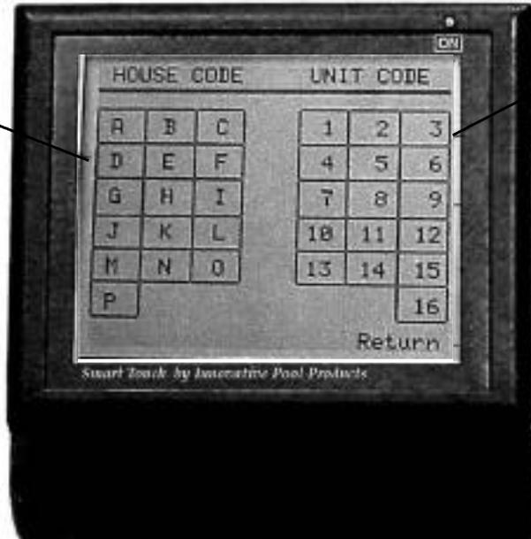
Set the unit code for standard PLC devices on Aux 7 - 13. The Smart Touch system used 1 entire house code.
