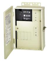
hese Control Centers feature an all-weather enclosure and contain a 4 circuit breaker base, an equipment grounding bar and a mechanical or electronic timer mechanism. The circuit breaker base accepts interchangeable type breakers made by a number of different manufacturers. In addition, the enclosure has provision for installing additional switches or GFCI receptacles on the side and inside.
