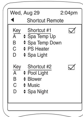
7. After assigning the button functions, mark the buttons with the labels provided.
