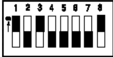
The ON position is shown with the black area facing upward.
