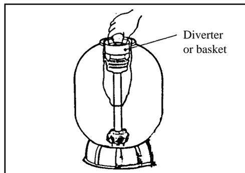
2. Place standpipe cover on standpipe to prevent entrance of any sand. Standpipe cover is either a plastic cap or waxed corrugated assembly found in misc. parts bag or separately in carton. Some filters may already have standpipe cover installed on standpipe and diverter removed and located in misc. parts bag.
