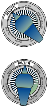
Fig. 10: Valve settings to lower pool water level. Stop pump before changing valve position.
