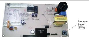
the pilot flame current using a bar graph and numerical display. A signal of less than 4 indicates a weak flame signal and may require service. Refer to Section 5 – Troubleshooting for possible causes and corrections.
