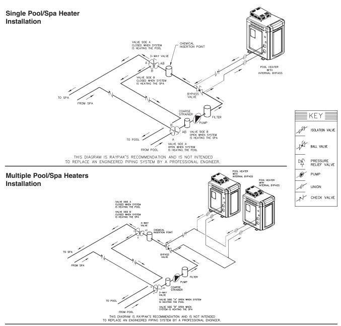
The heater requires water flow and positive pressure to fire and operate properly. It must therefore be installed downstream of the discharge side of the filter pump. A typical installation is plumbed as follows:
