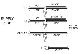
The heater must be electrically grounded and bonded in accordance with local codes, or, in the absence of local codes, with the latest edition of the National Electrical Code, ANSI/NFPA 70. (Canada - Canadian Electrical Code, CSA C22.1, Part 1 and Part 2.)
