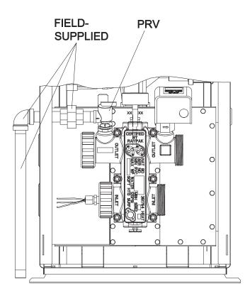
**NOTE:** To avoid water damage or scalding due to valve operation, drain pipe must be connected to valve outlet and run to a safe place of discharge. Drain pipe must be the same size as the valve discharge connection throughout its entire length and must pitch downward from the valve. No shut-off valve shall be installed between the relief valve and the drain line. Valve lever should be tripped at least once a year to ensure that waterways are clear.
