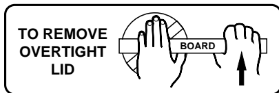
Figure 5 – Use a pry bar or board as shown to remove tight lid. Do not use a pry bar to tighten lid.
