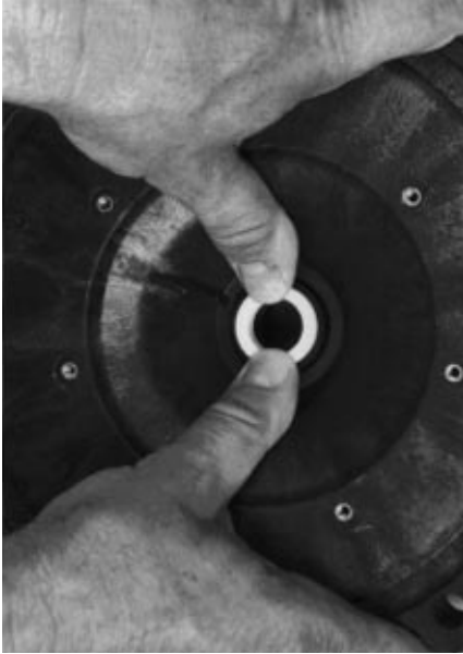
Figure 5: Press seal into heat sink in seal plate
