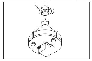
Replace the measuring cup with the appropriate sized measuring cone: A, B or C.
