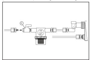
Cut the tubing to the proper length to attach to the male adapter in the pipe on the pressure side of the filter (D below). Avoid hose kinks and leave a little extra length of tubing. Hand tighten the tube nut.
