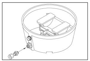
Apply teflon paste to the pipe threads on the check/flow valve and install it hand tight. The valve should be in the vertical position as shown. Do not over tighten.
