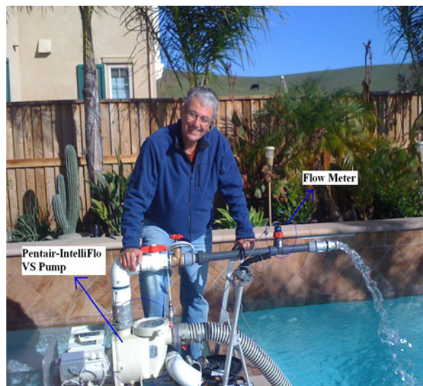
Figure 4. Hydraulic Cleaner Test Setup
