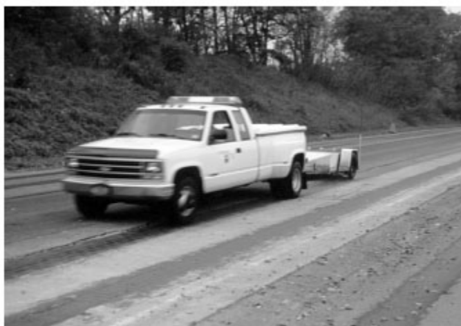
Figure 4. ASTM E 274 Test Equipment consists of a truck and trailer assembly. A tire within the trailer is towed at a given speed, locked, and skidded across water dispensed on the pavement in front of it.
