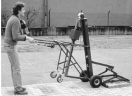
Figure 3. (below) Non-motorized equipment used to set a small layer of pavers. Figure 4. (right) Motorized equipment with a mechanical clamp.
