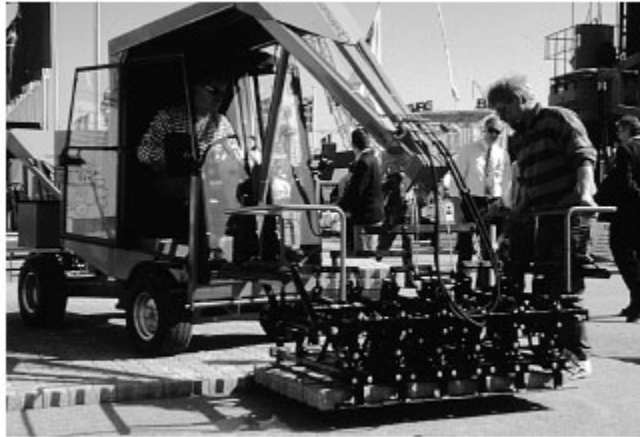
Figure 3. (below) Non-motorized equipment used to set a small layer of pavers. Figure 4. (right) Motorized equipment with a mechanical clamp.
