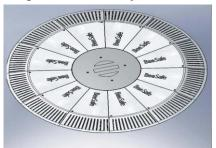
Model #: Bee Safe 46" dia. X 2" high retrofit for 8" dia., 10" Size: dia, 9" square, 12" square & some 18"sq. 146.25 sq. in. Open area: Floor Wall Flow rate (GPM): 792 none Velocity rate (FPS): 1.74 Single/Multiple: PVC 7140 Material: Testing Lab: NSF Notes: Weighs 90 lb.
