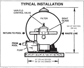
NOTE: If rigid return piping is used, installation of a piping union is recommended for ease of future servicing.
