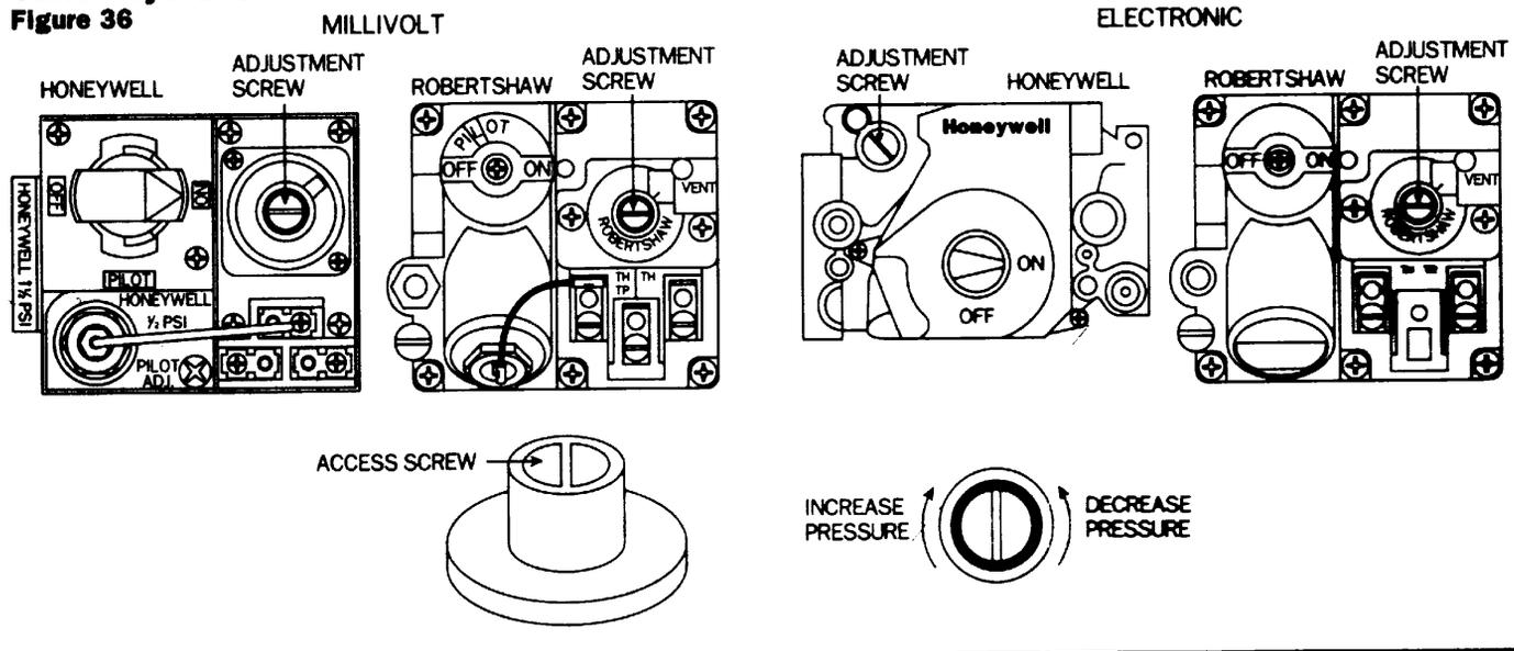
7. If the gas pressure does not meet the above requirements the regulator must be adjusted.
