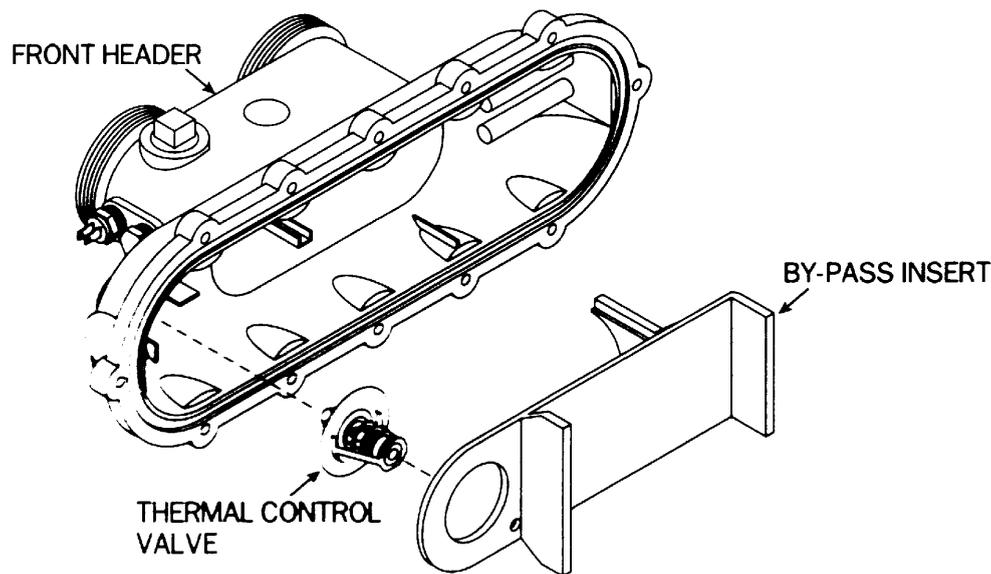
contacts. If the valve sticks closed, too much water will flow throughout the heat exchanger causing condensation to occur. Either situation may result in insufficient heating of the pool or spa.
