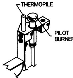
9. Push in control knob all the way and hold in. Push the spark ignitor button several times to light pilot. Continue to hold the control knob in for about one (1) minute after the pilot is lit. Release knob and it will pop back up. Pilot should remain lit. If it goes out, repeat steps 5 through 9.
