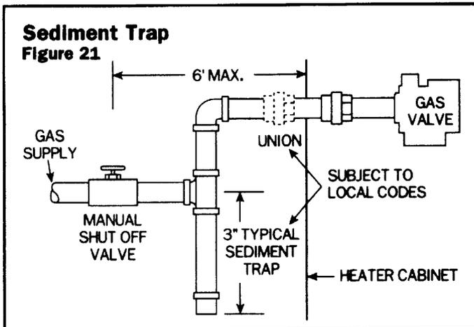
**Do not use flexible appliance connectors on any gas connections unless the connector is A.G.A. approved for outdoor installation, is marked with the BTUH capacity (which must be equal to or greater than the heater rated input), and the type of gas (Natural or LP) to be used.**
