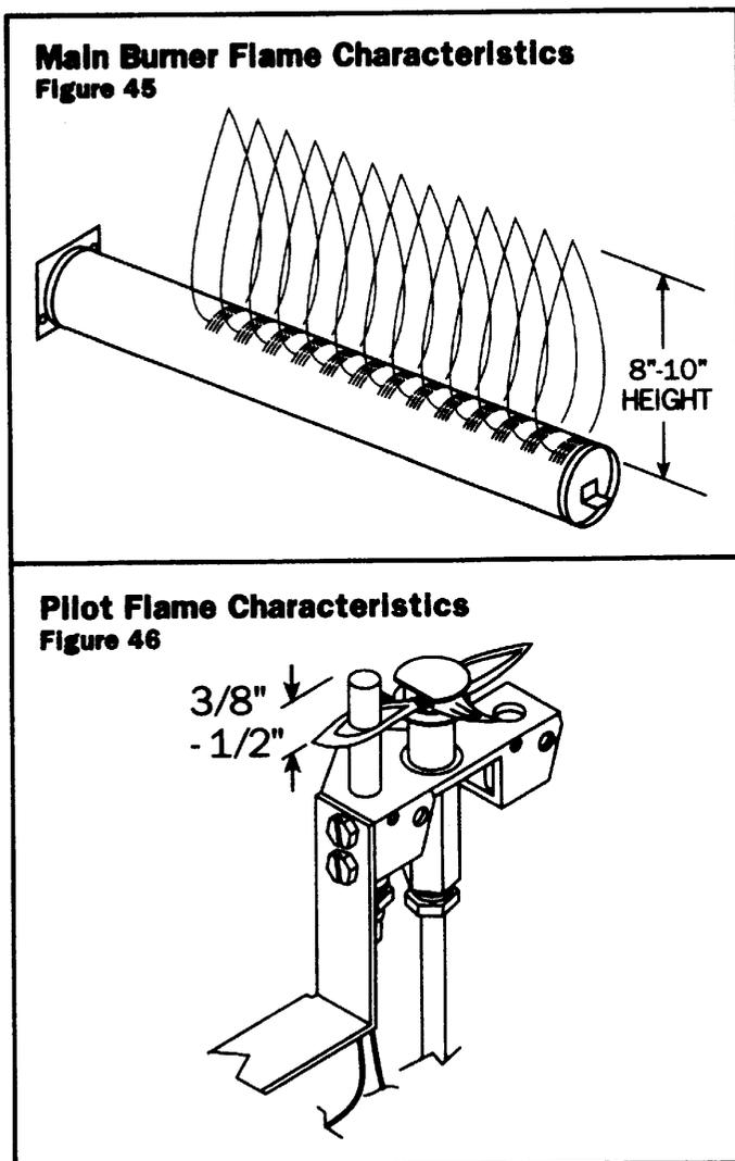
All burners should be brushed with a wire brush and be free of lint, dust and spider webs before each season of use. Burners with damaged ports must be replaced. See Figure 46 for pilot flame characteristics (millivolt heater only).
