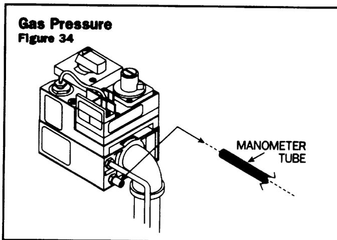
5. Turn on water system and start heater following the lighting instructions on the label inside the cabinet. If there is more than just the pool/spa heater connected to the gas supply line, turn each of those appliances on while testing the heater.
