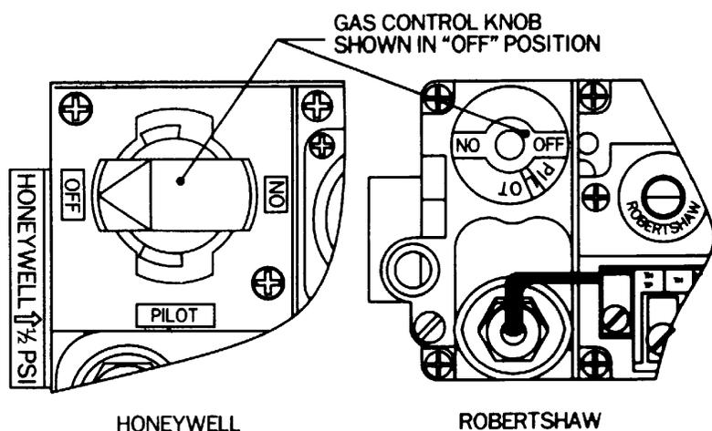
7. Find pilot - follow metal tube from gas control. The pilot is beside the burner tube to the extreme left.
