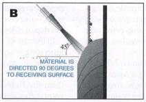
Proper shotcrete-application techniques are important in avoiding problems with vanishing-edge weir walls. It's vital, for starters, for the operator to know to avoid 'shadowing' and creating voids on the back side of the rebar (A). It's also critical that the material be shot at the appropriate angle and in ways that
