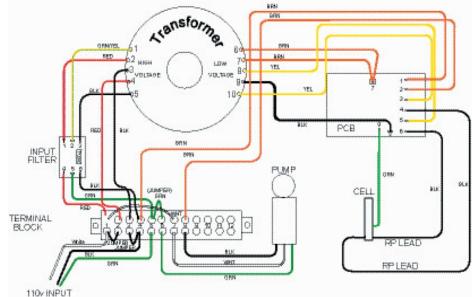
110v WIRING DIAGRAM
