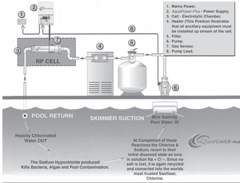
**Water may flow ONLY in the direction specified on the cell.**
