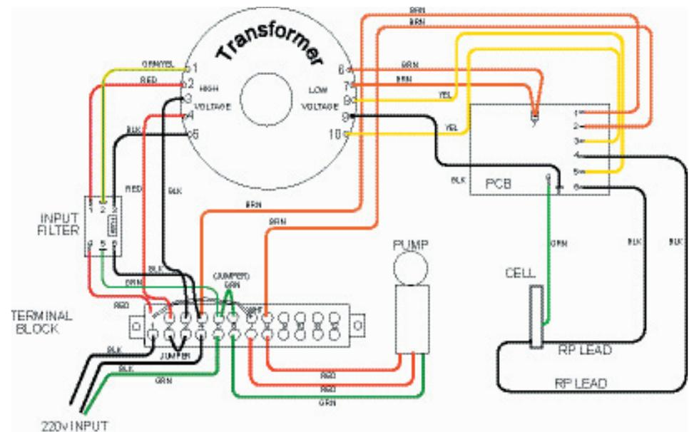
220v WIRING DIAGRAM
