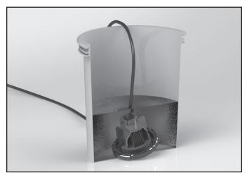
A foaming action will begin, which is caused by scale (calcium carbonate) being dissolved from the plates. If foaming action does not begin, the cell does not need to be cleaned (STOP THE CLEANING PROCESS - go to the step 10). Otherwise allow the cell to remain in the solution until the foaming has stopped (approximately 5 - 10 minutes).
