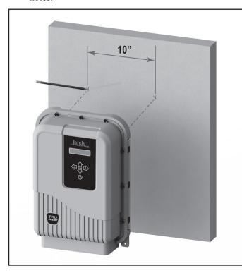
Drive the screws into the holes and hang the Power Pack from the top two holes of the backplate.
