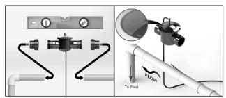
Make the appropriate cuts in the pipe where you 2. will be installing the cell. The gap between the cuts should be 6 inches.
