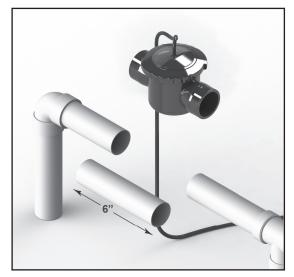
Remove the cell from the housing and plumb the housing into the pipe, making sure that the flow indicator arrows on the housing match the flow direction of the water. Pipes must be clean and dry before gluing.
