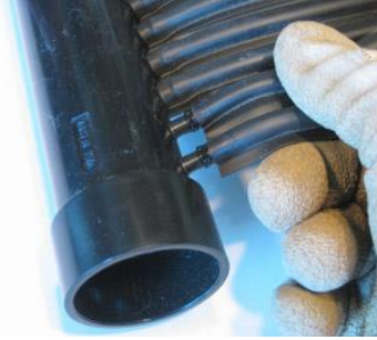
Pushing fin-tubing onto header 2 tubes at a time.
